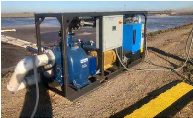
Exhibit 1-26. Nanobubbles Generator Unit - Courtesy of Moleaer
