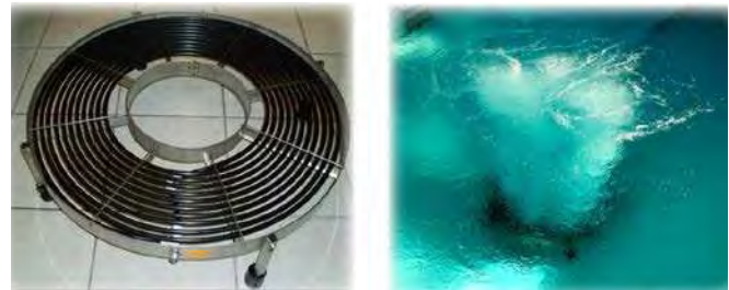
Exhibit 1-24. Installation of Aeration Modules with Buoys – San Dieguito Reservoir, Courtesy of ADS
