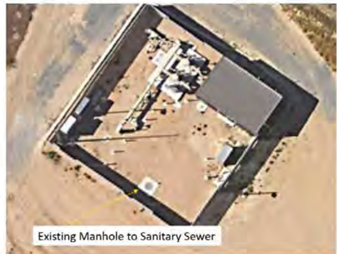
Exhibit 1-20. Syphon Reservoir Strainer Facility Existing Connection to the Sanitary Sewer
