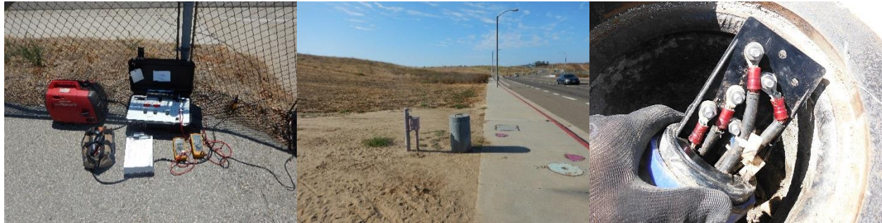
"Attenuation" Continuity Test Method Setup
