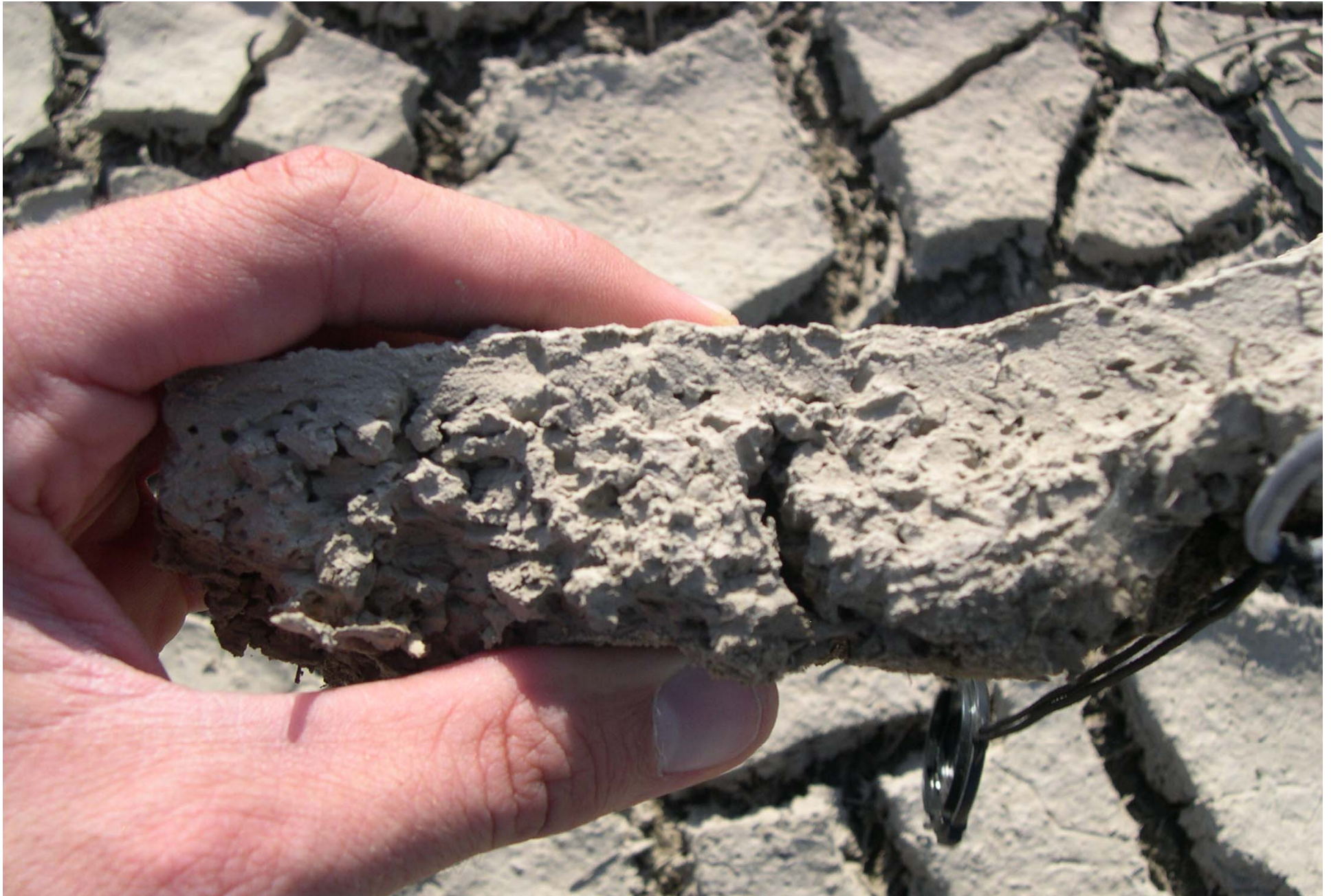
Photo 7b (36N): Basin No. 1 mud-cracks; thin mud-cake ~5 mm thick caps silty sediment; shallow soil shows evidence of biological activity
