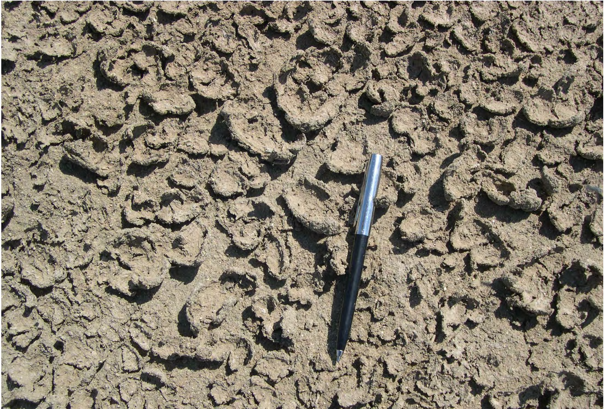
Photo 38b (10A): Basin No. 19 mud/bio-chips ~2-5 cm in length and ~1-4 mm thick overlying sandy silt sediment
